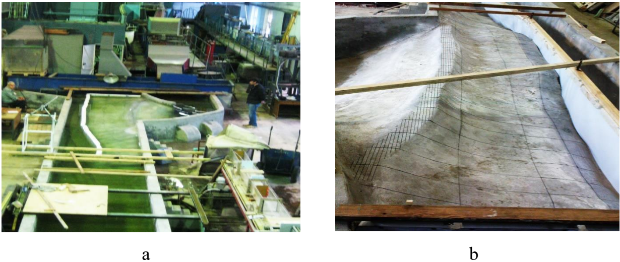
Fig. 1. Experimental stand (a) and relief of the bottom in front of the entrance section of the jet-directing screen (b).
